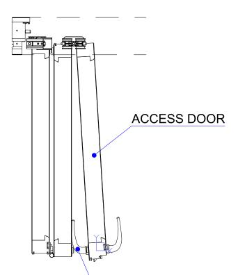
STANDARD HANDLE COLLIDES WITH ADJACENT DOOR AND PREVENTS THE ACCESS DOOR FROM FOLDING OPEN FULLY PARALLEL
