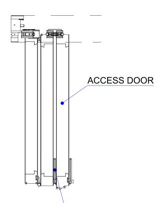
LOW PROJECTION HANDLE ALLOWS ACCESS DOOR TO FOLD OPEN FULLY PARALLEL
