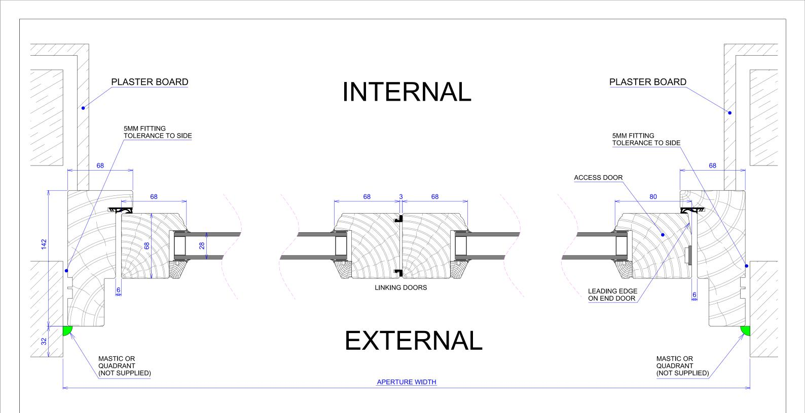
THE DOORS SHOWN ARE ODD AND ALL STACK TO THE LEFT (NO RIGHT DOORS). IF THE DOORS ALL STACKED TO THE RIGHT THE ACCESS DOOR AND THE LEADING EDGE WOULD BE THE OPPOSITE HAND TO THOSE ABOVE.
