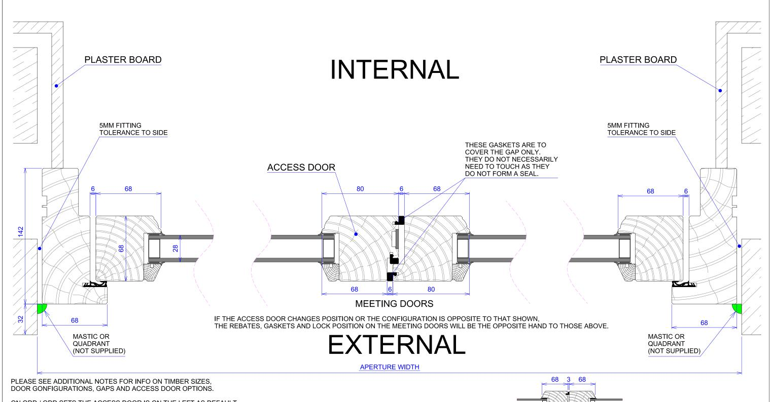
ON ODD / ODD SETS THE ACCESS DOOR IS ON THE LEFT AS DEFAULT. IT CAN BE CHANGED TO THE RIGHT DOOR UPON REQUEST.
